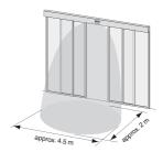
Installation height 2200 mm / angle of detection field  $30^{\circ}$ Antenna position:
